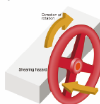
Shearing – a finger put through the spokes of the wheel will be sheared off
